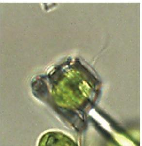
The basket trap: These algae are only 10 micrometers in size. They use two flagella at the front to move, similar to a swimmer's breaststroke, which made fixing them in traps without inhibiting their movement a challenge. The team experimented with four different-sized structures before selecting this final one. Credit: *Small* (2024). DOI: 10.1002/smll.202402923
