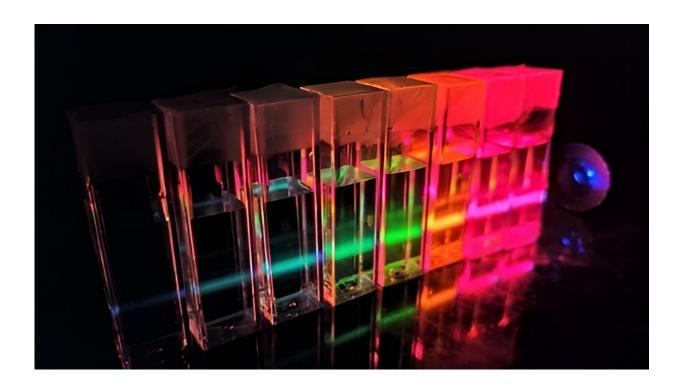
Cadmium telluride (CdTe) quantum dots of different sizes emitting light in response to excitation by UV laser. Credit: Pedro Felipe Garcia Martins da Costa
