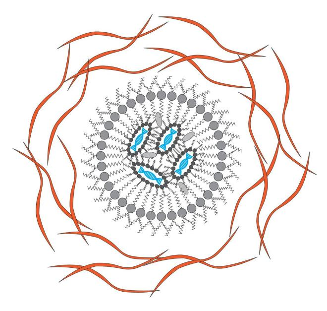
Schematic representation of a nanoparticle with a layer of sugar-glycerin (orange), a protective shell from lipids (grey) and enclosed DNA tracers (blue). Credit: Functional Materials Laboratory
