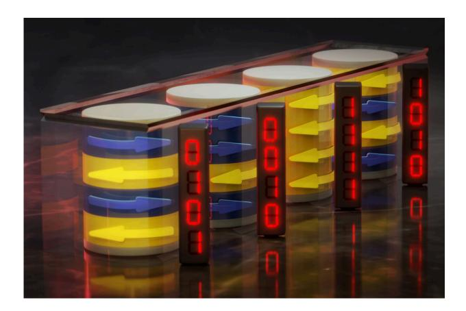
Information is stored by the depth-dependent direction of magnetization in the domain walls. By systematically varying these directions, researchers can encode different bit sequences within a cylinder domain. Credit: Helmholtz Association of German Research Centres
