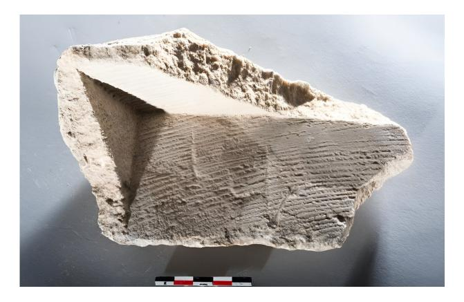
Carbonate fragment from the Barbegal mills, formed on wood of the mill machinery, with imprints of wood and traces of woodworking. Credit: Philippe Leveau
