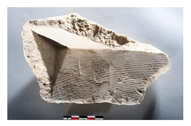
Carbonate fragment from the Barbegal mills, formed on wood of the mill machinery, with imprints of wood and traces of woodworking. Credit: Philippe Leveau
