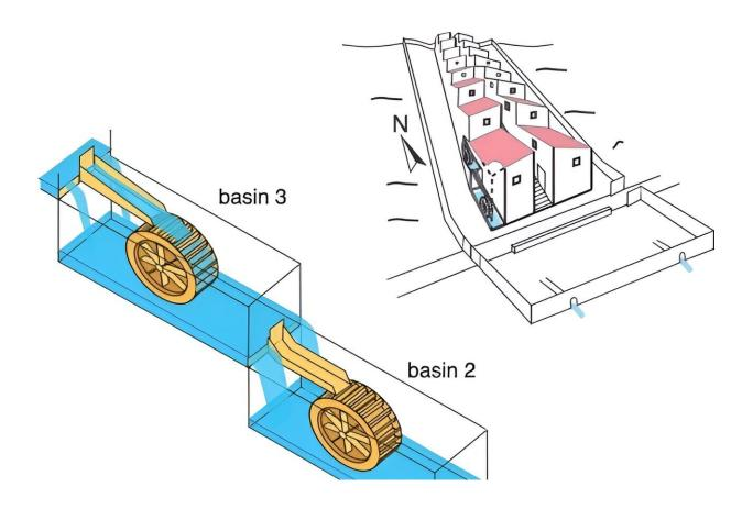
Sketch of the Barbegal mill complex with three water basins with mill wheels and water flumes. The lower basins probably had elbow-shaped flumes. Credit: Cees Passchier
