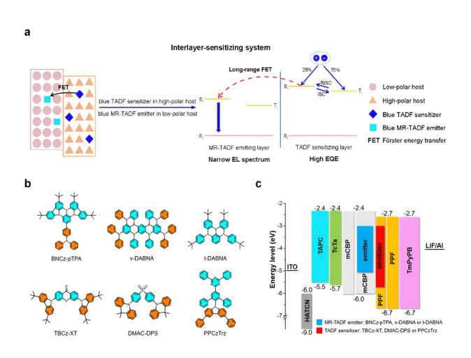
a, Schematic illustrations of interlayer-sensitizing system for blue MR-TADF emitters. b, Molecular structures of MR-TADF emitters and TADF sensitizers employed in the interlayer-sensitizing configuration. c, Device configuration of interlayer-sensitized hyperfluorescence devices. Credit: Jianghui Wang, Peng Zou, Letian Chen, Zhentao Bai, Hao Liu, Wen-Cheng Chen, Yanping Huo, Ben
