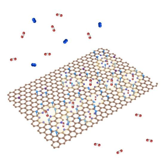
A schematic of porous graphene hosting pyridinic N (shown as purple spheres) at the pore edges. The resulting membrane is highly selective to  $CO_2$ . Credit: Dr. Kuang-Jung Hsu.
