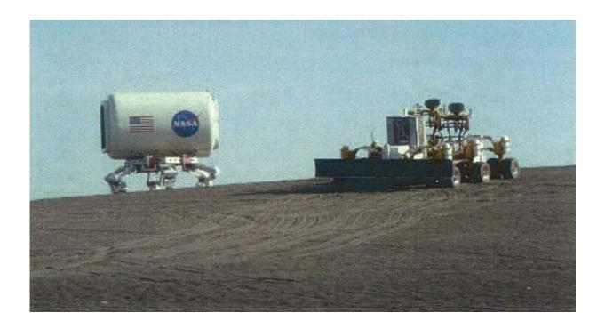
Chariot rover with LANCE attachment undergoing testing at the Moses Lake test site. Credit: Mueller et al.
