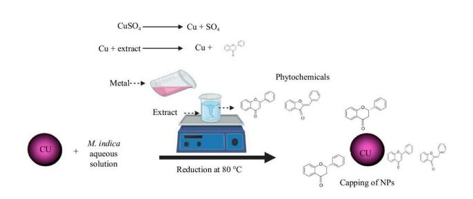
Proposed hypothetical picture of the reduction mechanism of copper sulfate by the aqueous leaf extract solution of M. indica on a hot plate at 80 °C for 4 h at 200 rpm. Credit: *Fruit Research* (2024). DOI: 10.48130/frures-0024-0015
