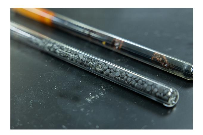
Some of the components of the chalcogenide glass stored in airtight vials where they are later processed at UCF's Glass Processing and Characterization Laboratory. Credit: Antoine Hart
