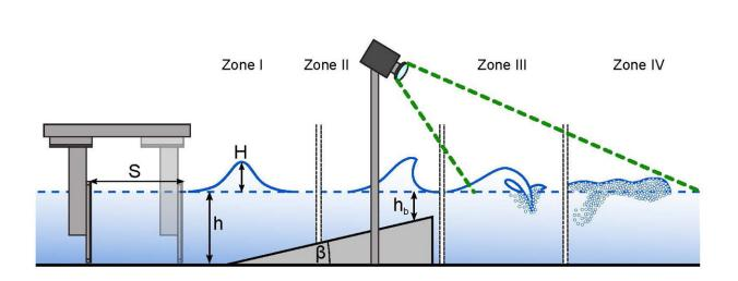
A wave channel experiment used a zoom lens camera and a custom Python script to process imagery of four different zones: wave generation, shoaling and breaking, air detained by a plunging jet of water, and air trapped at bores where water level rises rapidly. The study provided essential insights into the physical and chemical impacts of microplastics at the air-water interface. Credit: Jotam Bergfreund
