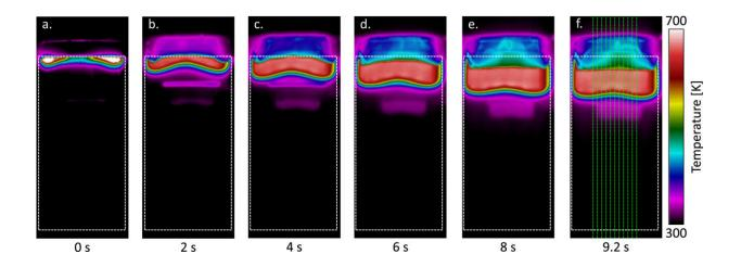
IR sequence of a µg experiment at 100 mm/s opposed flow, 75 kPa, and 28.3 %  $O_2$ . The sample contours are highlighted by white dashed lines. f. The evaluation lines used for the evaluation of the propagation rate are shown with green dotted lines. Credit: *Proceedings of the Combustion Institute* (2024). DOI: 10.1016/j.proci.2024.105358
