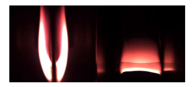
The image shows an ignited acrylic glass sheet during a microgravity experiment in the Drop Tower Bremen (left: sideview; right: front view). Credit: Florian Meyer, ZARM, University of Bremen
