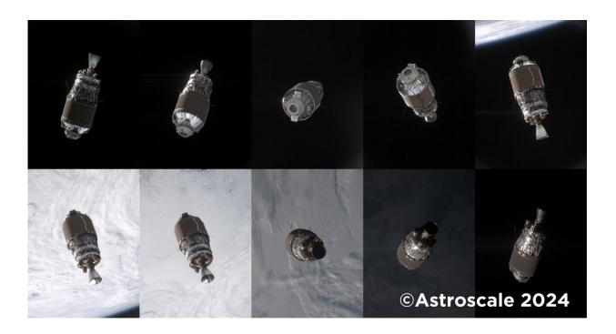
Figure 1: Images of the target space debris taken during the fly-around observation on July 15th 2024. The order of the images progresses from top left to bottom right. Credit: JAXA
