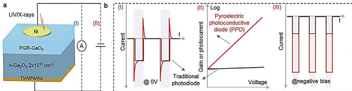
Schematic of the PPD based on PGR-GaOX film and its photoresponse compared to traditional photodiode. Credit: Prof. Long Shibing's team
