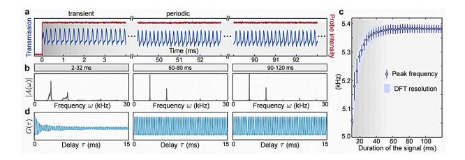
Establishment of the long-range temporal order. a. Single quenching dynamic of a time crystal b. Fourier transform of the oscillations for different time windows. c. The peak frequency of oscillation gradually stabilizes to a constant over time. d. The autocorrelation function (ACF) of time crystals for different time windows. Credit: Dr. Xiaoling Wu
