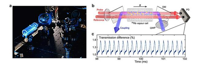
a. Photo of the team's experimental setup, with the luminated vapor cell at room temperature without cooling or heating. b. Schematic of the experimental setup, where a probe beam overlaps with a counterpropagating coupling beam in a room-temperature 85Rb-vapor cell and establish EIT. c. A typical oscillating time crystal signal. Credit: Dr. Xiaoling Wu
