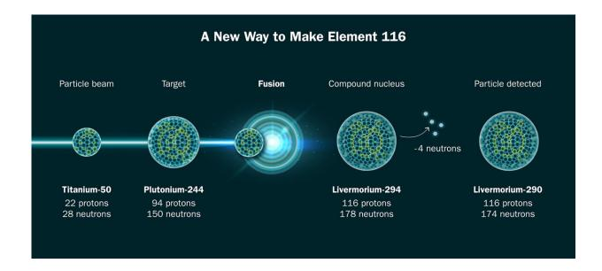
To make element 116, researchers fused isotopes of titanium and plutonium. Credit: Jenny Nuss/Berkeley Lab
