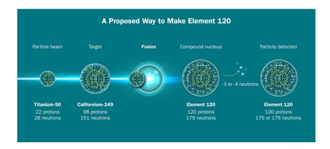
To make element 120, researchers want to fuse isotopes of titanium and californium. Credit: Jenny Nuss/Berkeley Lab
