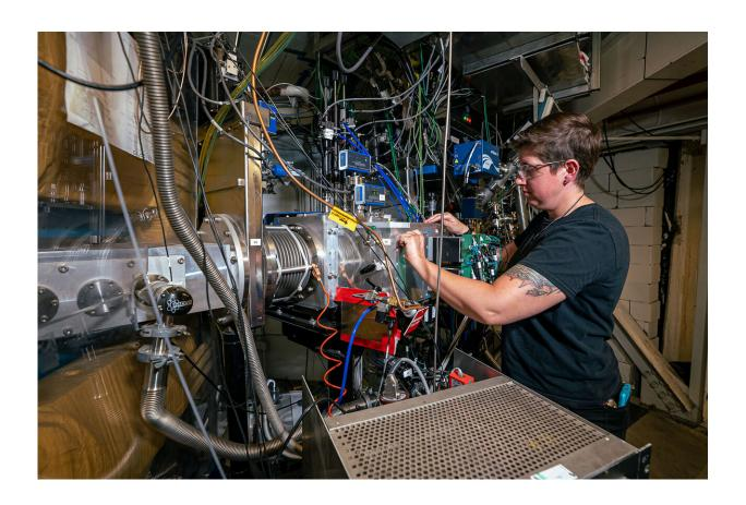
Scientist Jacklyn Gates at the Berkeley Gas-filled Separator used to separate atoms of element 116, livermorium. Credit: Marilyn Sargent/Berkeley Lab
