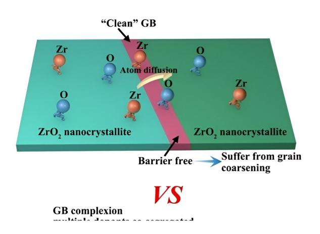
In un-doped  $ZrO_2$ -SiO<sub>2</sub> system, the GBs between  $ZrO_2$  nanocrystallites were clean without dopant segregation. When heating the material, Zr and O atoms could easily cross the GBs, resulting in grain coarsening. In comparison, when multiple dopants were added to the material system, GB complexions with multiple dopants co-segregated were formed. The GB complexions acted as a barrier for atom diffusion, which effectively hindered grain coarsening. The
