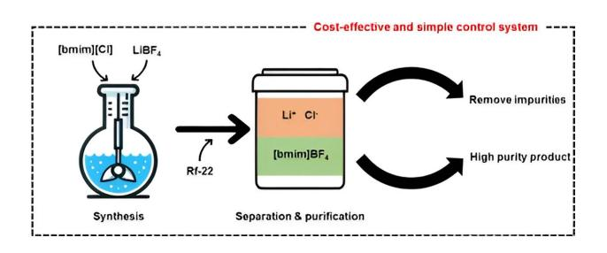
Schematic of ionic liquid synthesis and purification process. Credit: *Industrial & Engineering Chemistry Research* (2024). DOI: 10.1021/acs.iecr.4c01218
