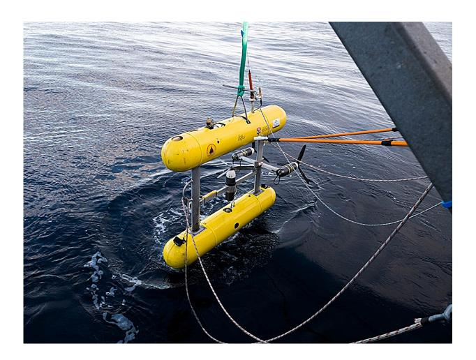
Autonomous underwater vehicle being deployed. Credit: IMOS
