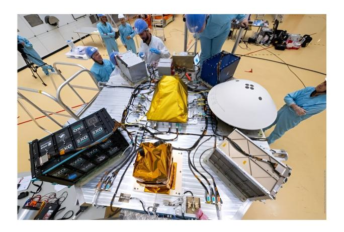
Final tasks to integrate the EXOpod Nova module with the launcher Ariane 6. Credit: ESA
