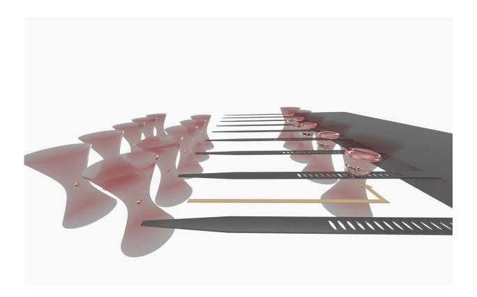
A rendering of the atom-nanophotonic interface designed by Bernien Lab members, which will allow the construction of large quantum systems which can be easily scaled up. Credit: Bernien Lab, Pritzker School of Molecular Engineering
