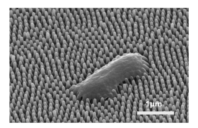
Scanning electron microscope image of a *Pseudomonas aeruginosa* bacterium, destroyed by nanopillars, on a cicada wing. Scale bar is 1 micrometer. Credit: Yutao Chen. Credit: Yutao Chen.
