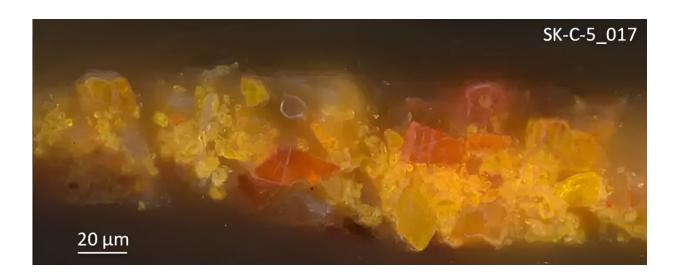
Cross section of paint sample SK-C-5\_017 as seen through a light microscope. It shows various crystals of yellow, orange and red pigments of which the precise composition was established using a combination of electron microscopy, Raman spectroscopy, and X-ray powder diffraction. Credit: Rijksmuseum.
