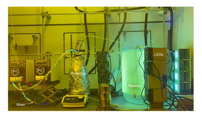
In-house circulation-flow reactor (picture taken with a yellow filter for clarity). Credit: *Nature Chemistry* (2024). DOI: 10.1038/s41557-024-01560-7
