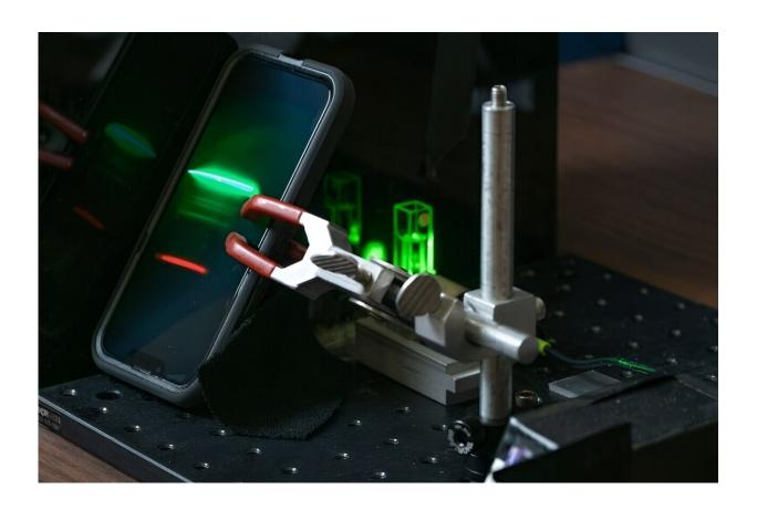
A smartphone records the Raman spectrum of an unknown material (an ethanol solution, in this case) for further analysis. Credit: Texas A&M University Engineering
