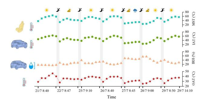
Measured material surface temperature, in-cabin air temperature, in-cabin relative humidity, and out-cabin air temperature during the field tests. MST, material surface temperature; IAT, in-cabin air temperature; IRH, in-cabin relative humidity; OAT, out-cabin air temperature. Credit: *PNAS Nexus* (2024). DOI: 10.1093/pnasnexus/pgae243, https://academic.oup.com/pnasnexus/article/3/7/pgae243/7717707
