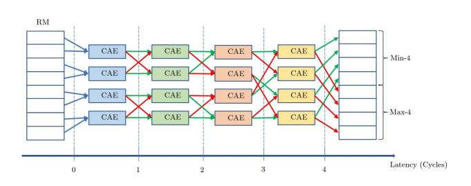
Block diagram of a pipelined MSS8 corresponding to an MSS built for ???=3. The green (red) arrows represent the smaller (larger) of the two outputs of the respective CAE units. Credit: *Scientific Reports* (2024). DOI: 10.1038/s41598-024-60319-9
