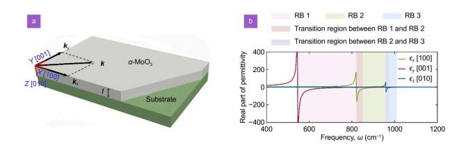
(a) Schematic of  $\alpha$ -MoO<sub>3</sub>/substrate heterostructure, where the substrate is SiC or Au. (b) Real parts of the components of the dielectric tensor of  $\alpha$ -MoO<sub>3</sub> along the principal directions. The Reststrahlen bands are shaded in different colors. Credit: *Opto-Electronic Science* (2024). DOI: 10.29026/oes.2024.240002
