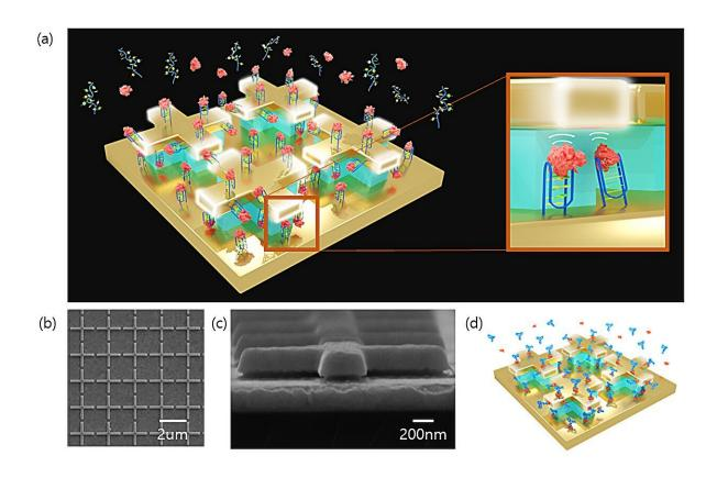
(a) Schematic of a vertical nanogap biosensor for label-free thrombin immunoassay, with thrombin-binding aptamer (TBA) immobilized on the metamaterial absorber (MA) structure. Top (b) and side views (c) of the SEM image. (d) Illustration of protein A/G and IgG bilayer-incubated MA structure. Credit: *Biosensors and Bioelectronics* (2024). DOI: 10.1016/j.bios.2024.116436
