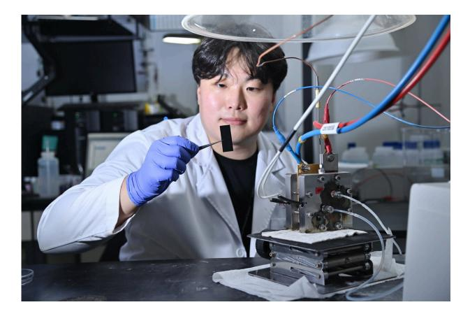
An electrode with a molybdenum MXene catalyst transferred onto an electrolyzer device. The cathode element, one of the key components of a hydrogen production device, is being held. Credit: Korea Institute of Science and Technology
