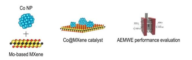
Overall concept of catalyst design using MXene as an electrocatalyt support and its utilization as an electrode for an anion exchange membrane water electrolyzer. Credit: Korea Institute of Science and Technology
