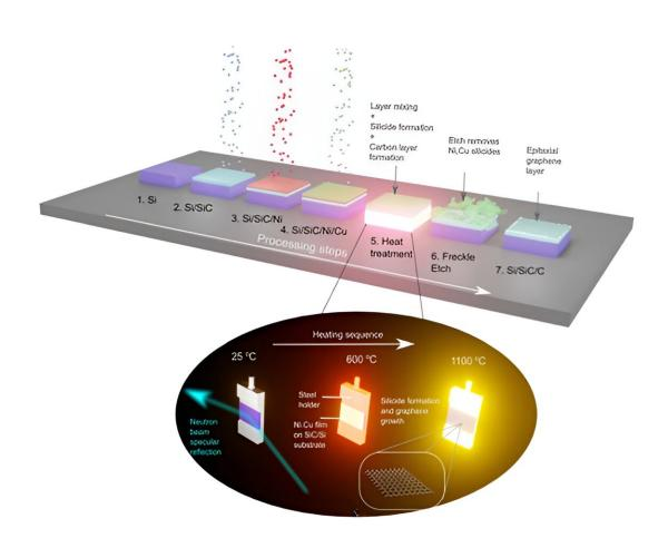
Schematic of the Ni/Cu catalytic alloy-mediated EG synthesis on 3C–SiC on silicon. Credit: *RSC Advances* (2024). DOI: 10.1039/D3RA08289J
