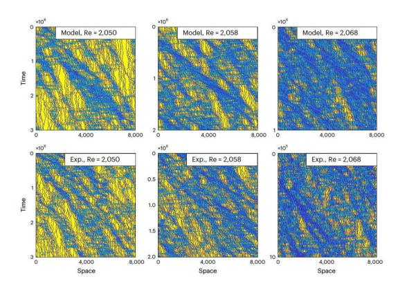
Trajectories in time traced out by turbulent puffs as they move along a simulated pipe and in experiments, with blue regions indicate the puff "traffic jams." The images on the left are closer to the laminar-turbulent transition than those on the right, so one can clearly see the traffic jams melt away as the directed percolation transition is approached. Credit: Nigel Goldenfeld / UC San Diego
