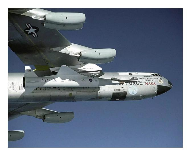
NASA's B-52B launch aircraft cruises to a test range over the Pacific Ocean carrying the third and final X-43A vehicle, attached to a Pegasus rocket, on Nov. 16, 2004. Credit: NASA
