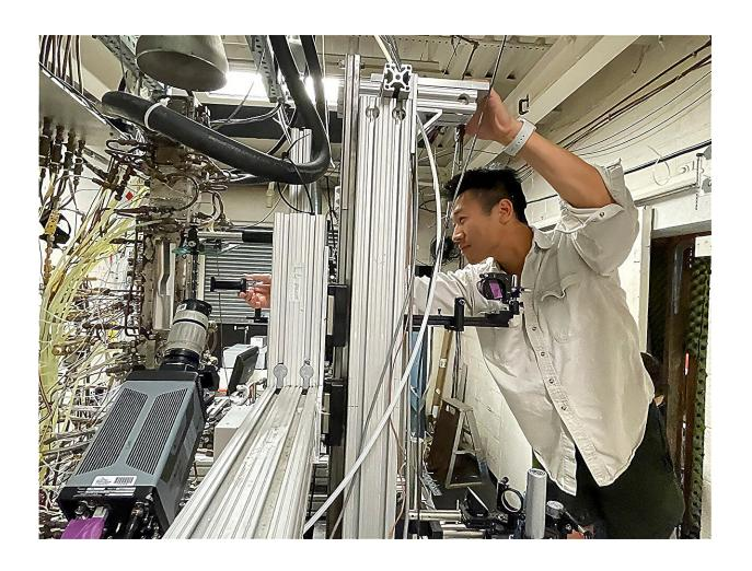
Doctoral student Max Chern takes a closer look at the wind tunnel setup where University of Virginia School of Engineering and Applied Science researchers demonstrated that control of a dual-mode scramjet engine is possible with an optical sensor. Credit: Wende Whitman, UVA Engineering
