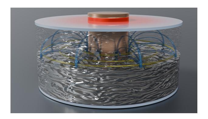
A schematic 3D visualization of gallium (transparent in this schematic) and mercury layers, showing the thermoelectric poloidal currents (blue) and magnetic field (yellow). Credit: Christophe Gissinger
