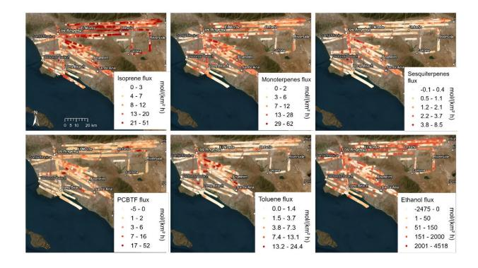
Maps of the fluxes of six VOCs that were important for SOA formation and OH reactivity measured along the flight tracks. Data from all nine flights is shown here. Values are 2 km running averages downsampled to 100 m. Credit: *Science* (2024). DOI: 10.1126/science.adg8204
