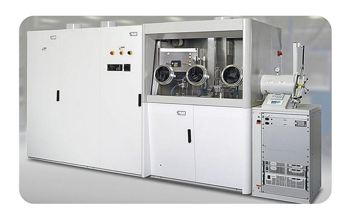
Metal-Organic Chemical Vapor Deposition (MOCVD). Credit: Electronics and Telecommunications Research Institute(ETRI)
