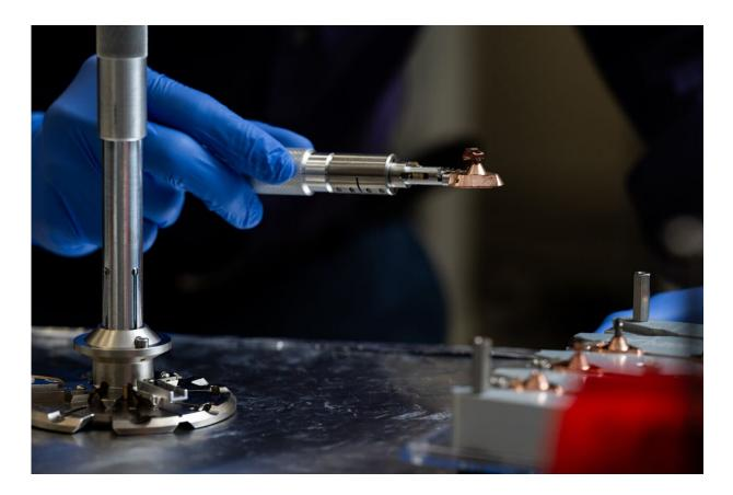
Microscopic samples of complex metal alloy are placed on a sampling vessel to enter the atom probe tomography instrument. Credit: Andrea Starr | Pacific Northwest National Laboratory
