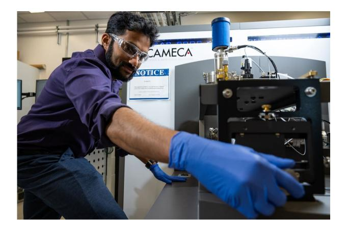
Materials scientist Arun Devaraj works at an atom probe tomography instrument at Pacific Northwest National Laboratory. This precision instrument can show the placement of atoms in tiny samples of materials, such as metal alloys. Credit: Andrea Starr | Pacific Northwest National Laboratory
