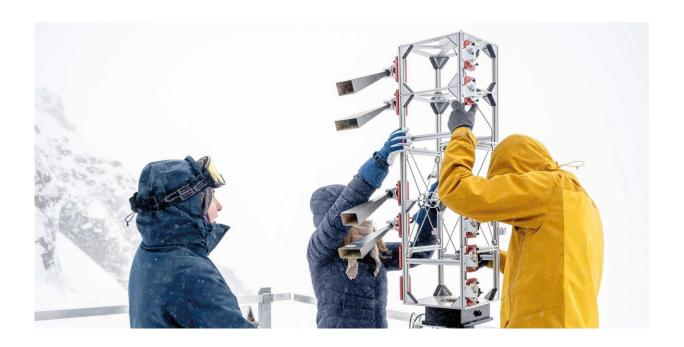
The researchers position the radar – and its horn antennas – on a sturdy base. Credit: ETH Zurich / Daniel Winkler
