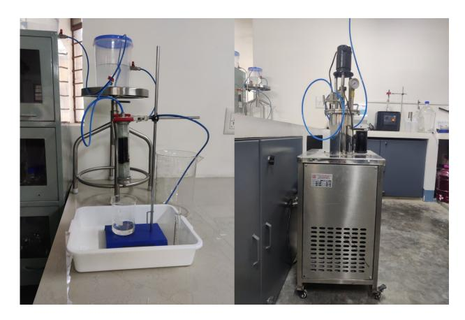
The adsorbent stage (left) and remediation stage (right) in the pilot system in the lab. Credit: Sustainable Separation Solutions (S3) Lab, CST, IISc
