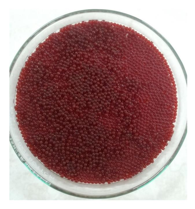
Close-up view of the adsorbent beads. Credit: Sustainable Separation Solutions (S3) Lab, CST, IISc
