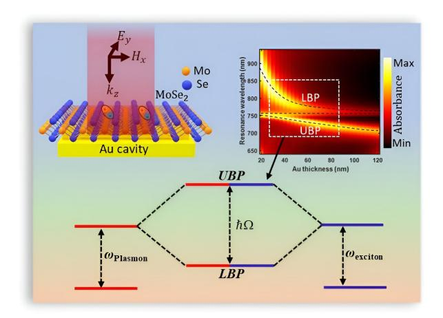
Top: (Left) Schematic illustration of monolayer MoSe<sub>2</sub> on top of Au cavity at normal incidence with polarization along the y-axis, and (Right) its corresponding absorption spectrum mapping with varying Au thickness. Insert (bottom): Schematic representation of strong coupling between a plasmon mode
