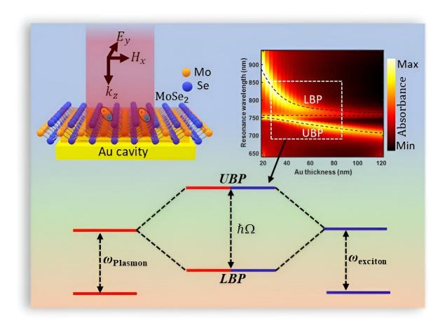
Top: (Left) Schematic illustration of monolayer MoSe<sub>2</sub> on top of Au cavity at normal incidence with polarization along the y-axis, and (Right) its corresponding absorption spectrum mapping with varying Au thickness. Insert (bottom): Schematic representation of strong coupling between a plasmon mode
