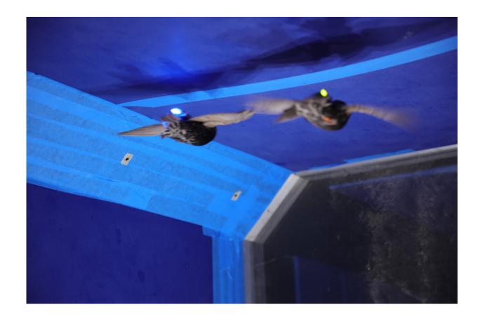
A view from below of two European starlings flying together in a wind tunnel while wearing inertial measurement units with a colored LED marker. Credit: Siyang Hao
