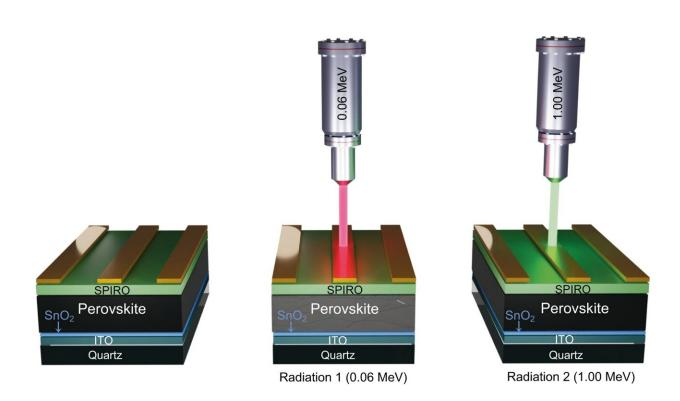
Dual dose irradiation experiments. Irradiation of the PSC with a NIEL-dominated 0.06 MeV proton beam (red) is followed by irradiation with a 1.0 MeV proton beam (green). By varying the fluence of the two radiation exposures, we selectively demonstrate how IEL participates in partial recovery of the solar cell performance after initial radiation damage. Credit: *Nature Communications* (2024). DOI: 10.1038/s41467-024-44876-1
