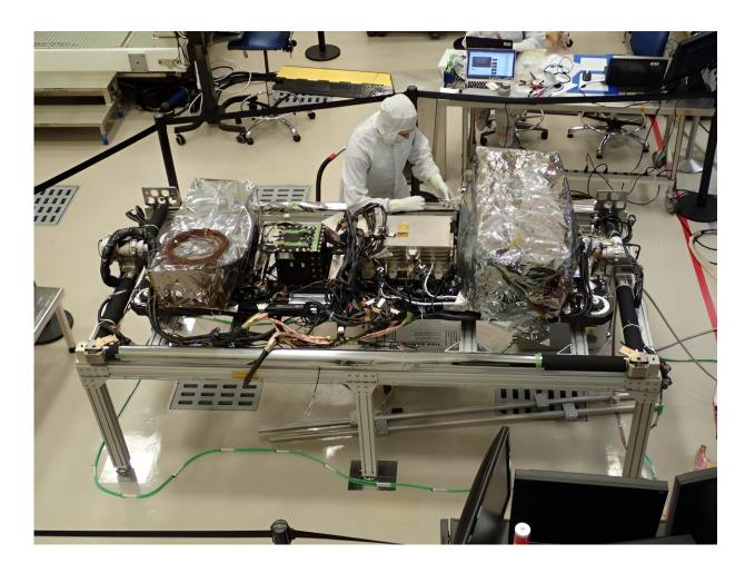
A technician installs an EXIS instrument onto the solar pointing platform of the GOES-T satellite, which launched in 2022. Credit: NOAA Satellites
