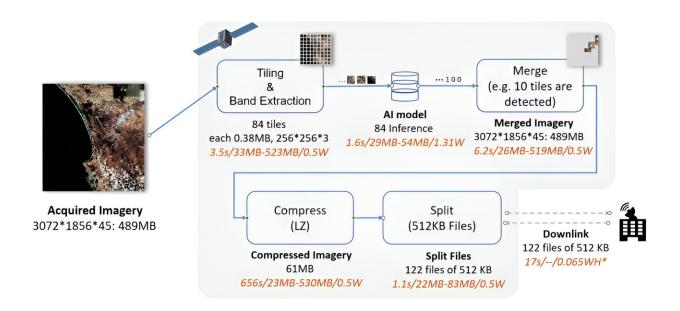
Simulation of the onboard smoke detection process using AI, detailing the steps of tiling, band extraction, AI model inference, image merging, compression, and file segmentation for downlinking, along with their respective time, memory, and power requirements. Credit: *IEEE Journal of Selected Topics in Applied Earth Observations and Remote Sensing* (2024). DOI: 10.1109/JSTARS.2024.3394574
