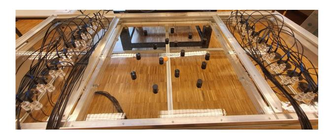
The experimental setup, with speakers and microphones at either end of a water tank, and vertical scattering objects at the center. Credit: EPFL/LWE CC-BY-SA 4.0
