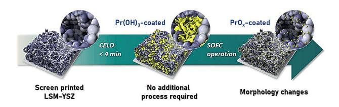
Schematic illustrations of the electrochemical coating process on LSM-YSZ electrode of SOFCs. Credit: Korea Institute of Energy Research (KIER)
