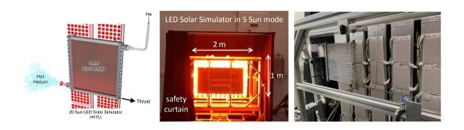
Image of the test set-up for the thermal shield. Credit: (2023). DOI: 10.2172/1960159
