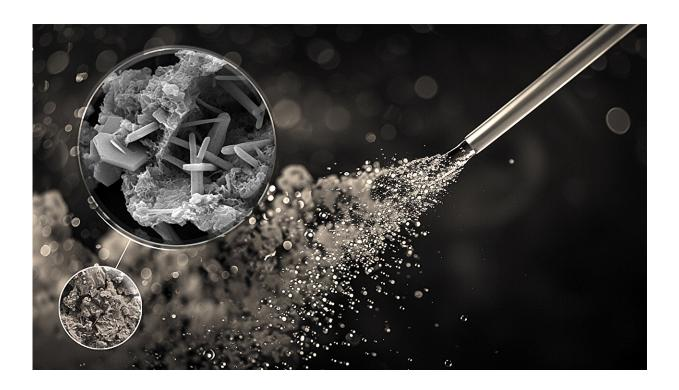
By using a carbonated — rather than a still — water-based solution during the concrete manufacturing process, engineers discovered a new way to store carbon dioxide. Credit: Alessandro Rotta Loria/Northwestern University
