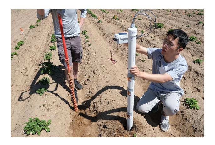
Soil science Ph.D. student Shuohao Cai places a sensing rod, which has multifunctional sensing stickers positioned to enable multi-depth measurements, in soil at UW-Madison's Hancock Agricultural Research Station to test the team's technology. Credit: Kuan-Yu.
