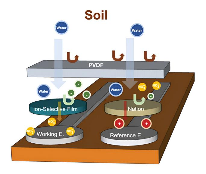
Schematic description of the working principle behind the open circuit
