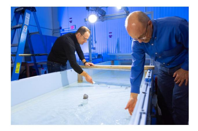
The team uses a video camera overhead and an object detection model to track the shiners' movements, as well as the water velocity, inside the flume. Credit: Douglas Levere/University at Buffalo
